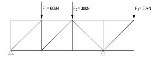
form diagram 1:100 force diagram  $1cm \triangleq 10kN$
