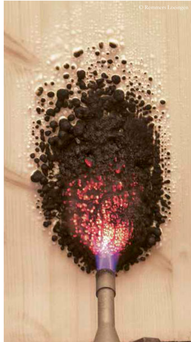
BESCHICHTET COATED (Fire coating)
