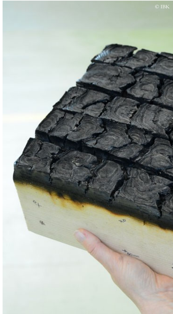
NATÜRLICH NATURAL (Protection with surface charring)
