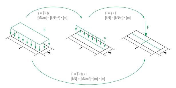
To convert area load  $\bar{s}$  to a point load F, we need to multiply  $\bar{s}$  with the width b and length l.
