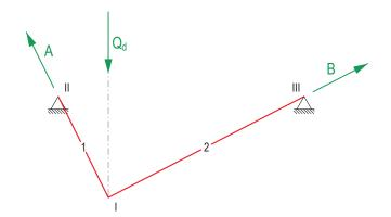
$Q_d = Q_k \cdot \gamma_Q$  $= 30 \text{ kN} \cdot 1.5$ = 45 kN
