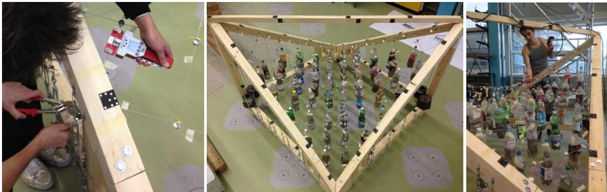
Figure 5: Prestress introduced through twenty external turnbuckles, measured with a portable tension meter and applied loads from 60 sand-filled PET bottles.
