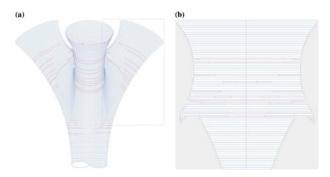
Fig. 10. a Courses for the four-directional minimal surface; and b knitting pattern for right branch (box) of the minimal surface
