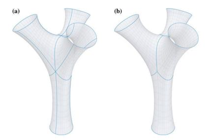
Fig. 9. a Patching of the surface for pattern generation; and b patches knit in one piece
