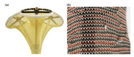
Fig. 11. a Physical prototype of minimal surface knit using the resulting knitting pattern; b short row features on knit prototype colourised for illustrative purposes
