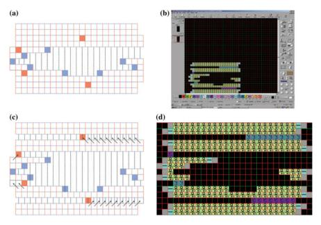
**Fig. 6. a** Resulting 2D pattern; **b** knitting pattern within SDS-one knitting machine software; **c** resulting knitting pattern showing the necessary transformations for knitting software; **d** resulting knitting pattern as represented in knitting software
