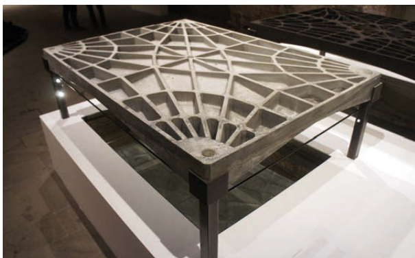
↙ FIGURE 7: Unreinforced rib-stiffened concrete funicular floor prototype
