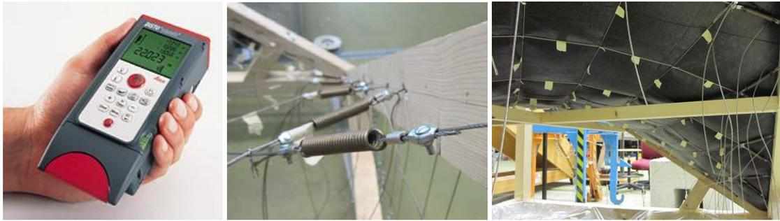
Figure 4: Measurement of first prototype; a Leica Disto Classic 5 laser metre for the geometry and springs for the forces.
