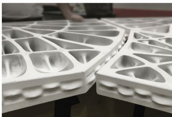
Block Research Group, Ribbed 3D-printed floor, Institute of Technology in Architecture, ETH Zurich, 2016
